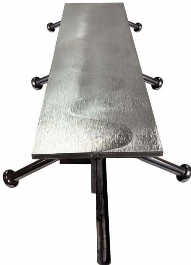
Conecto Sinus 06NC115 is heavy-duty joint profile for protecting and reinforcing joints in highly stressed concrete floors. Designed with a sinus wave, it ensures smooth, vibration-free travel for industrial forklift, regardless of tire size or hardness wheels. This innovative design minimizes noise and vibration and guarantees durability floor. It serves also as permanent formwork for concrete floors, offering robust edge protection and effective load transfer.
